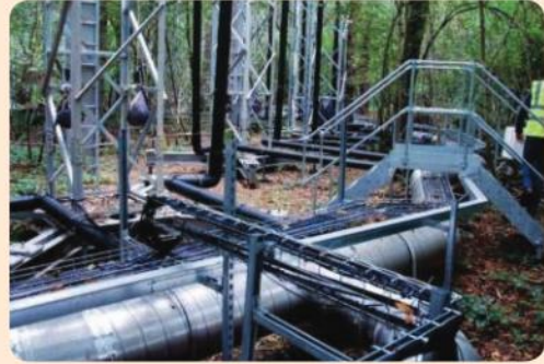
▲ The set-up used to raise the carbon dioxide concentration of an oak forest in Staffordshire (UK) from 400 to 550 ppm
